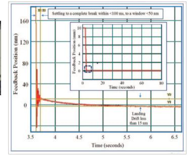
The motion profile reflects the position and velocity profile, reaching position stability at the end of the move command, settling to +/- 1 encoder count. The drift (position stability) is measured at <5nm per minute.
