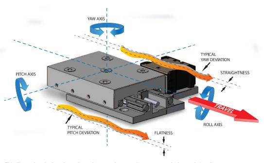
This illustration depicts the various elements that contribute to error. A given axis has linear errors, in the form of straightness & flatness and angular errors in the form of pitch, yaw & roll.
