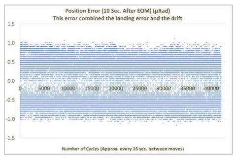
The graph above represents a test, simulating 5 years of operation service, moving 90°, 180°, 270°, 360° and back to home.
