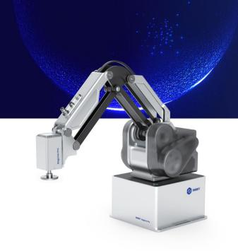
MG400 is a lightweight desktop robot with a footprint smaller than one piece of A4 paper. Designed to be flexible to deploy, easy to use, and safe to collaborate, MMG400 makes automation affordable and accessible for diversified and small-batch production scenarios. Featuring 750g payload, 440mm maximum reach, hand-held teaching and collision detection, MG400 truly fits perfectly for lightweight desktop applications and fast deployment in the production line.
